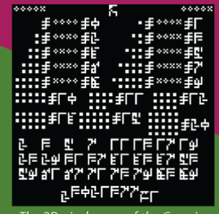
The 2D pixel array of the Cosmic Call message is resistant to alteration by noise as it travels through space due to its unique structure.
